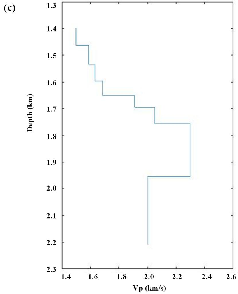
Fig. 4. (a) Ray diagram through the model. (b) The fit between the observed (red dots) and the calculated (blue lines) travel times. The time is reduced with a velocity of 8 km/s. (c) The P-wave velocity-depth profile obtained at the station of OBS7.
