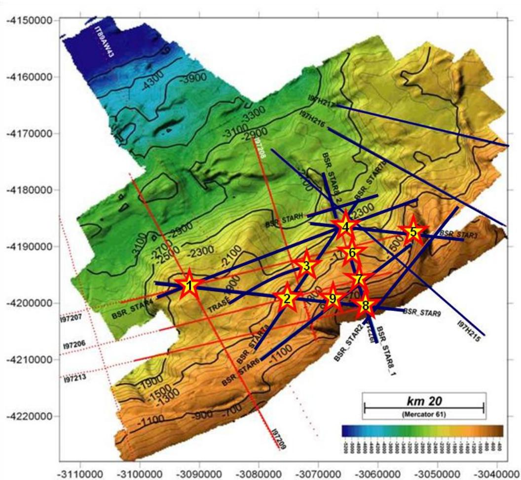
Fig. 1. Bathymetry map with the location of OBS (stars) and MCS data (solid lines)
