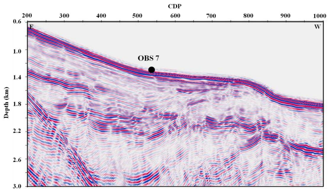
Fig. 2. A part of pre-stack depth migration section of MCS line I97214
