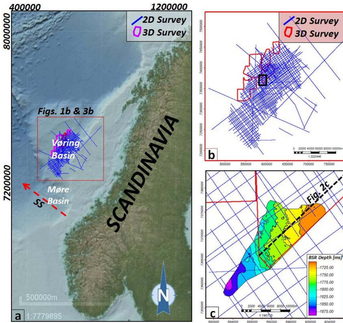
**Figure 1. Study Area** (a) Geographical location of the Vøring Basin, offshore Norway. (b) 2D and 3D seismic reflection dataset analyzed in this study, location shown in Figure 1a. (c) Spatial distribution of the gas hydrate related BSR mapped in the study area [25 ms TWT contour interval], location is shown by the black square in Fig. 1b. SS denotes Storegga slide and red dotted arrow indicates the transport direction.
