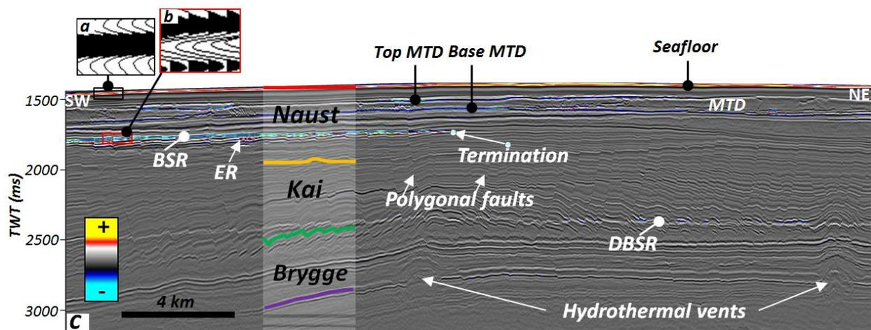
**Figure 2. BSR providing evidence for gas hydrate in the Vøring Basin** (a) Top left insert is a wiggle trace of the seafloor, note the opposite polarity when compared to the BSR in Fig.1b. (b) Wiggle trace of the BSR. (c) Seismic section showing the BSR and other fluid flow elements in the study area, location is shown in Fig. 1c. ER denotes enhanced reflection and MTD denotes mass transport deposit.
