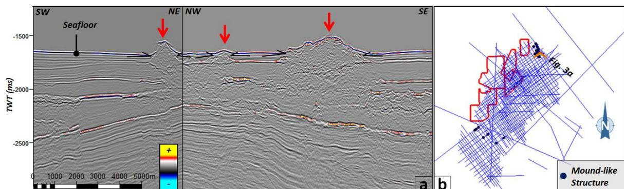
**Figure 3. Evidence of large-scale sediment remobilization in the Vøring Basin expressed as mound-like structures. (a) Seismic profile showing mounded structures indicated by the red arrows, location is shown in Fig. 3b. (b) Location of the mound-like structures mapped in the study area, for geographical location see Figure 1a.**
